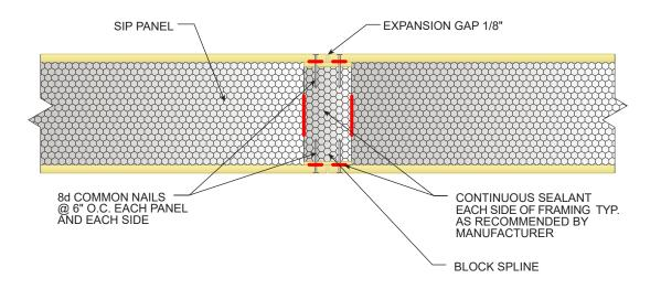
WALL-TO-WALL VERTICAL PANEL CONNECTIONS
